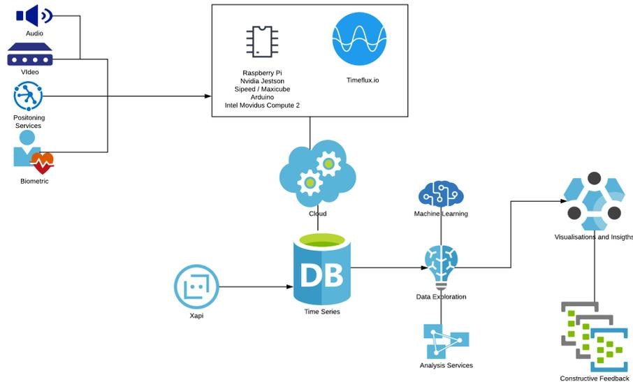
Figure 1: Conceptual Architecture of MBOX
